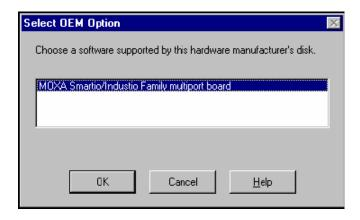
3. After the files have been installed, a configuration panel will open. This is where boards are installed, configured, and removed. If another board has already been installed on the system, it will already be listed. Windows NT does not automatically detect Moxa UPCI boards, so you will need to click Add for a newly installed board.
