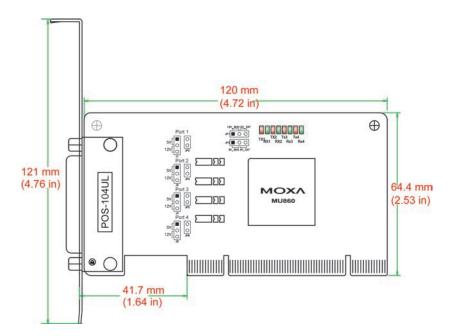
The onboard jumpers are used to specify the pin 9 power signal for each serial port.
