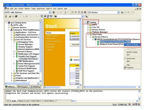
6. After adding Moxa Tech drivers into your OS Design, a new project is automatically added to your workspace. The project name is mxserce5. The project can be accessed from File View (View → File View). The mxserce5 project contains a number of files used to configure the drivers included in your OS Design.
