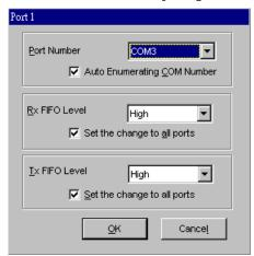
Select an **Rx FIFO Trigger** and **Tx FIFO Size**. The default Rx FIFO Trigger is 120 bytes (high level). The default Tx FIFO Size is 128 bytes (high level). Select **Set the change to all ports** to use this setting for all serial ports on the board.
