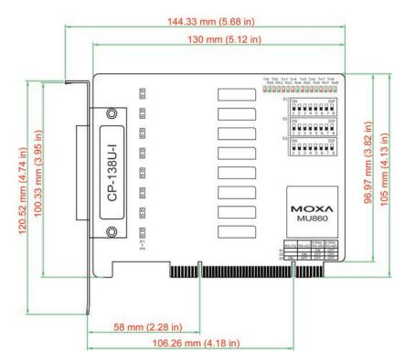
Onboard termination resistors can be activated individually for each serial port using jumpers JP1 through JP8. For CP-138U-I, JP1/2/3/4/5/6/7/8 corresponds to serial port 1/2/3/4/5/6/7/8, respectively. For CP-138U, JP1/2/3/4/5/6/7/8 corresponds to serial port 8/7/6/5/4/3/2/1, respectively. Short the jumper pins to activate the termination resistor; leave the jumper pins open to bypass the termination resistor.
