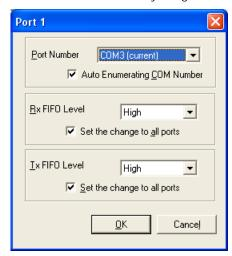
3. Select an **Rx FIFO Trigger** and **Tx FIFO Size**. The default Rx FIFO Trigger is 120 bytes (high level). The default Tx FIFO Size is 128 bytes (high level). Select **Set the change to all ports** to use this setting for all serial ports on the board.
