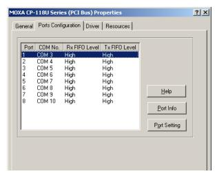
Under Port Number, select a COM number to assign to the serial port. Select Auto Enumerating COM
