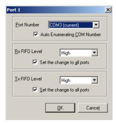
3. Select an Rx FIFO Trigger and Tx FIFO Size. The default Rx FIFO Trigger is 120 bytes (high level). The default Tx FIFO Size is 128 bytes (high level). Select **Set the change to all ports** to use this setting for all serial ports on the board.
