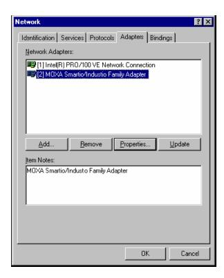
2. The configuration panel will open with a list of installed boards. Select your board and click **Property**. Up to 4 Moxa UPCI boards can be installed at a time.
