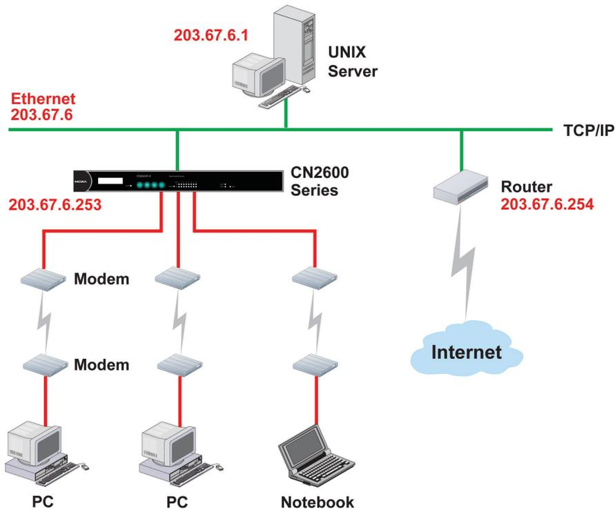
In this example, the Notebook PC dials into the CN2600 to request a connection to the Internet host at **210.48.96.9**, which is not on the local network **203.67.6.xxx**. This causes the CN2600 to act as a router and send the datagram to the default next-hop router, **203.67.6.254**. In this case, we should add the gateway IP address of **203.67.6.254** to the routing table to handle hops to **210.48.96.9**.
