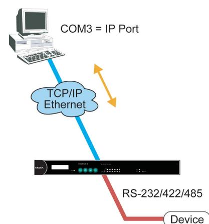
One of the major conveniences of using Real COM mode is that it allows you to use software that was written for pure serial communication applications. The Real COM driver intercepts data sent to the host's COM port, packs it into a TCP/IP packet, then redirects it through the host's Ethernet card. At the other end of the connection, the CN2600 accepts the Ethernet frame, unpacks the TCP/IP packet, and then transparently sends the data through the serial port to the attached serial device.
