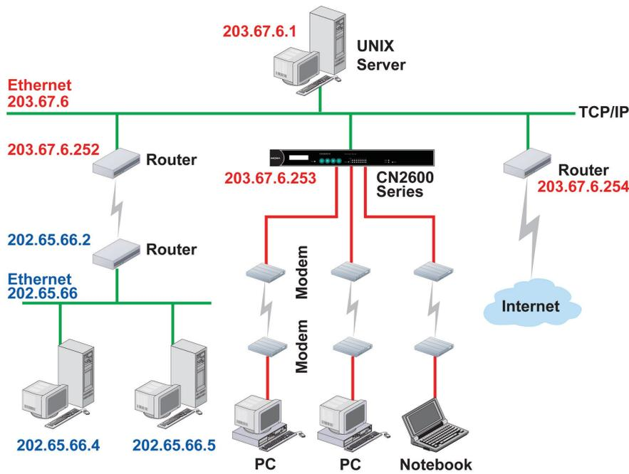
In this example, dial-in users can make requests to Intranet hosts **202.65.66.4** or **202.65.66.5**, which are on network **202.65.66.xxx** (located outside network **203.67.6.xxx**). You will need to add a route entry for the next-hop router, **203.67.6.252** that delivers requests to network **202.65.66.xxx**. The metric hop in this case is 2 route hops.
