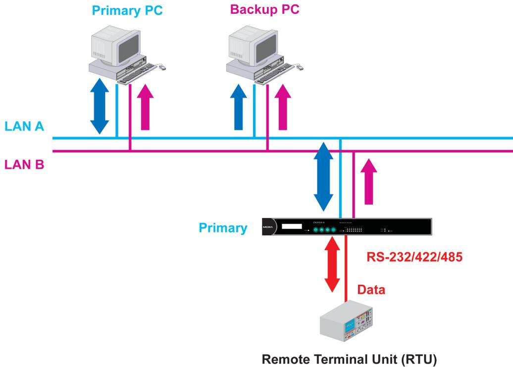
The DRDAS operation mode provides a highly redundant network structure that takes advantage of the CN2600's dual LAN ports, dual IP addresses, and dual MAC addresses. DRDAS uses a backup PC that is set up to take over when the primary PC fails.
