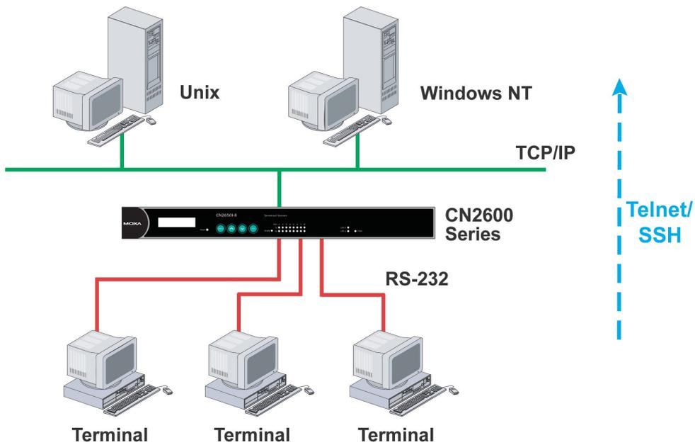
Terminal applications involve connecting terminals to UNIX or Windows servers over a network. A terminal connects to the appropriately configured serial port the CN2600, and the CN2600 transmits information to and from a UNIX or Windows server over the network through its Ethernet port. You may need to check with your network administrator to determine the appropriate terminal mode. All terminal modes support fast keys as used in many terminal applications.
