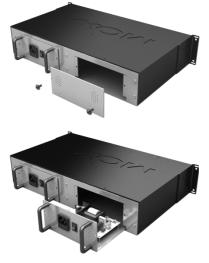
3. Where there is no plate on the chassis, slide the power supply module slowly and follow the installation guide in the chassis. Push the power supply module into the chassis till the end and ensure that the power supply module is firmly connected to the chassis.
